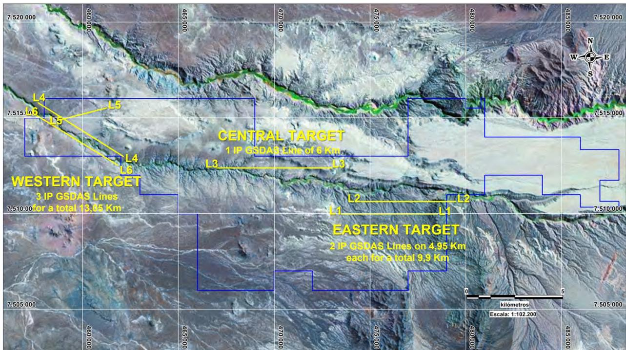
Figure 9-9. Location of the 6 completed Induced Polarization lines (L3 & L5 = 2D-IP; L1-L2 & L4-L6 = 3D-IP) over the three target areas at Tres Mariás – concessions outline in blue (see Table 9-1)(Alto Verde Copper, 2023).
