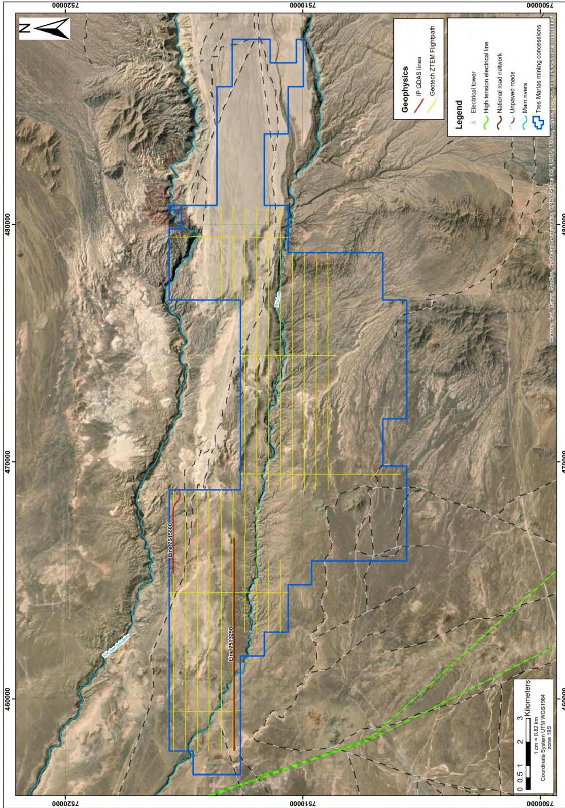
Figure 6-9. Flight lines (yellow) for the Geotech heliborne ZTEM and magnetics survey (2013) and ground lines (red) for the SouthernRock IP-MT survey (2015), along with the Property boundary and local infrastructure (information from Alto Verde Copper, 2023).
