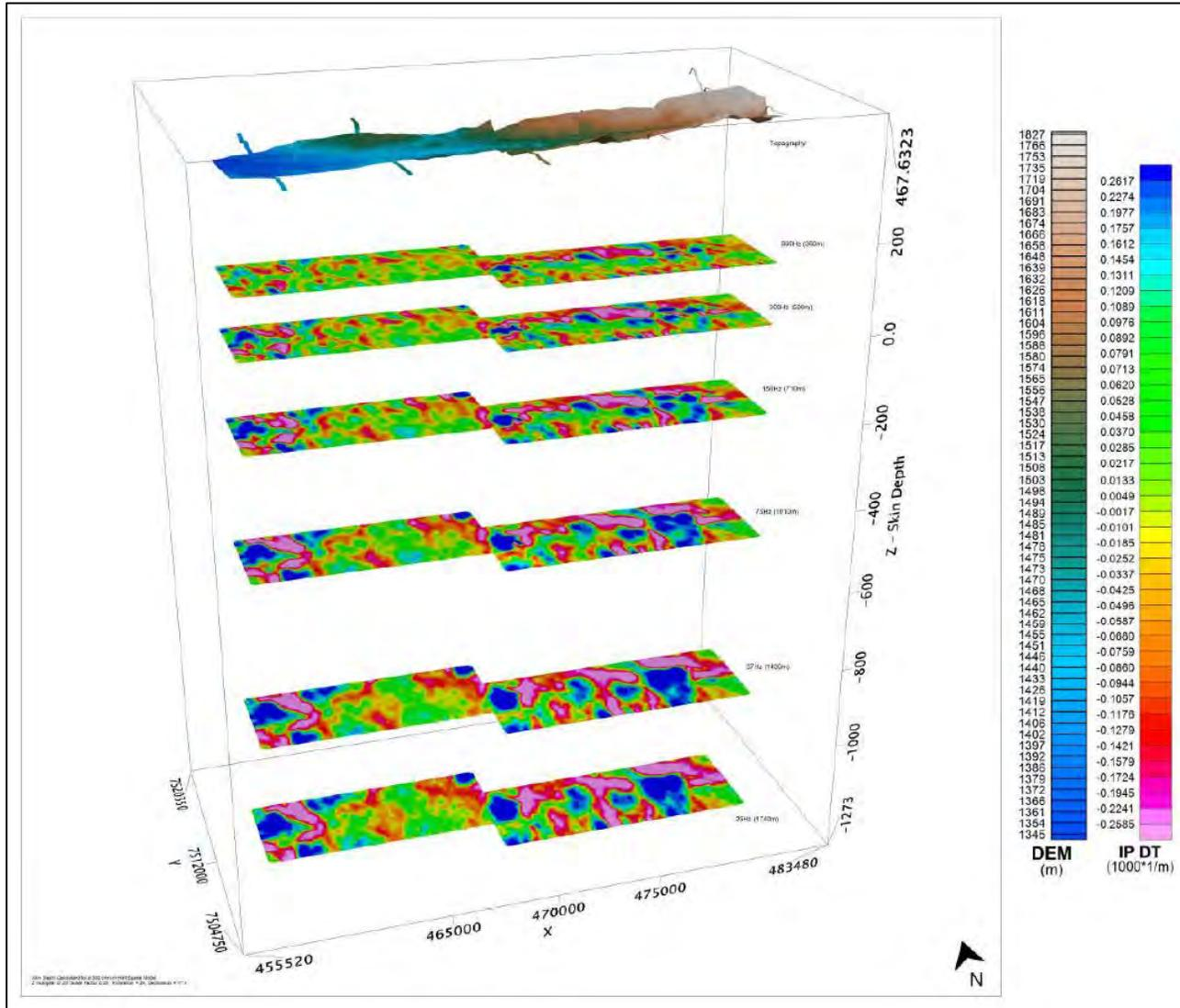
Figure 6-10. Isometric view of 3d inversions (ZTEM depth slices) showing In-Phase Total Divergence versus Skin Depth (25-600Hz) (Geotech, 2013).
