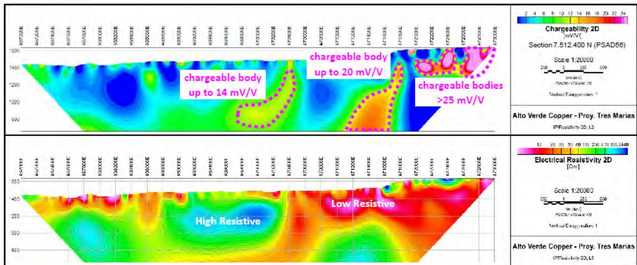
Figure 9-10. 2D chargeability (top) and resistivity (bottom) pseudosections for line L3 (Central Target), looking north (after Zamudio, 2021).
