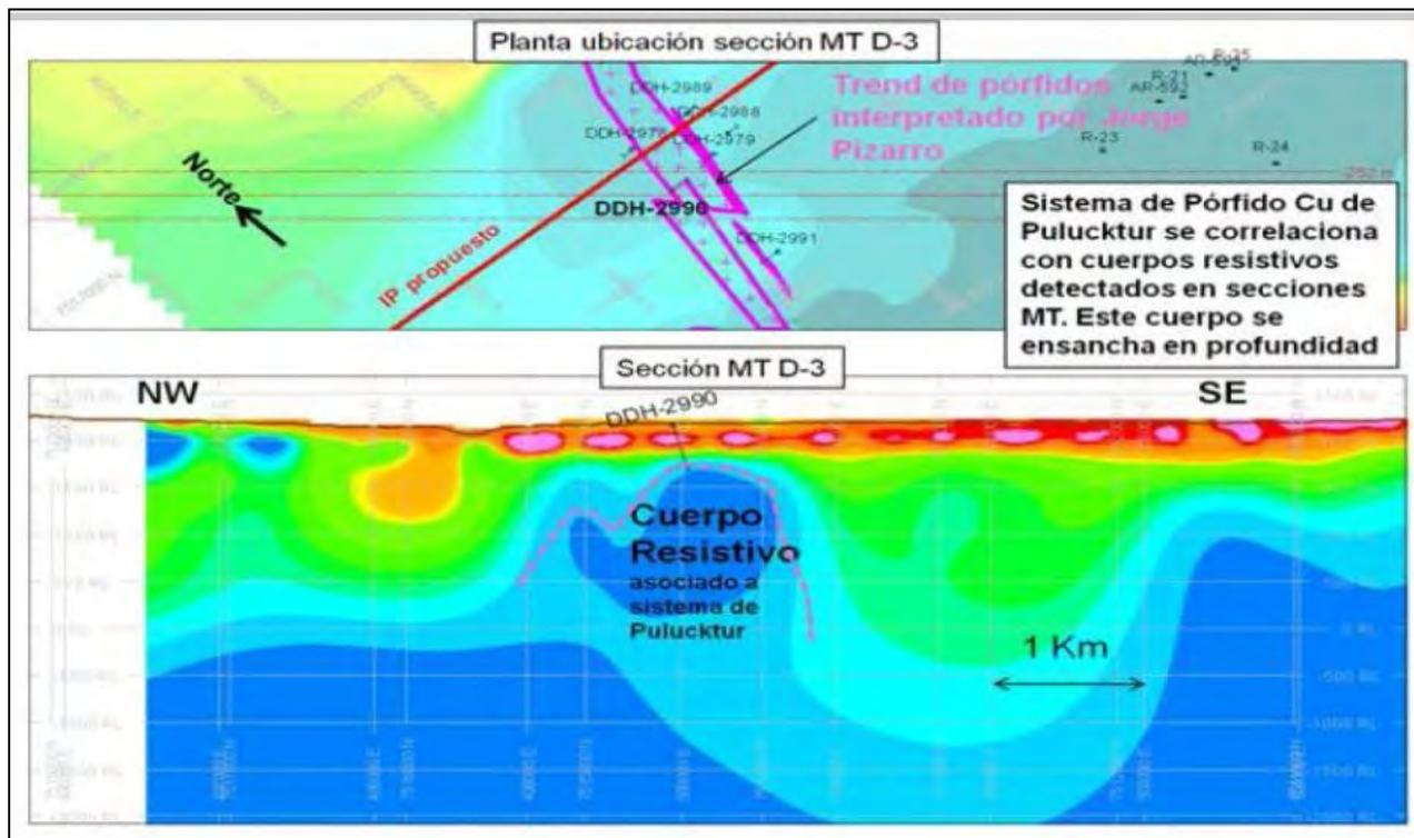
Figure 8-2. Geophysical cross-section of the analogous Codelco Opache deposit (Candia and Oviedo, 2016).
