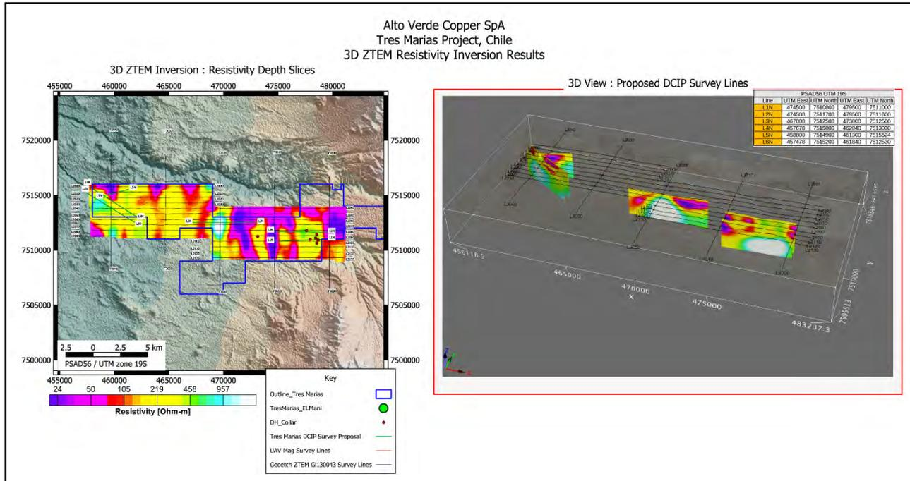
Figure 9-4. LEFT: Example Resistivity Inversion depth slice at 600 m vertical from re-processed 2013 ZTEM survey data. RIGHT: 3D view of Resistivity Inversion profiles along the planned IP survey lines planned for the ongoing 3D-IP survey (Alto Verde Copper, 2022).
