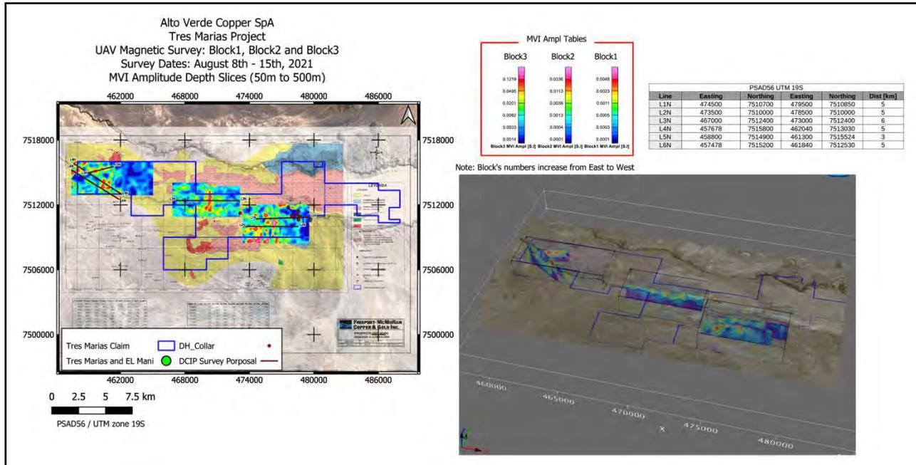
Figure 9-8. LEFT: Example of 3D Magnetic Vector Inversion (MVI) depth slices at 300 m vertical over the three target areas using UAV magnetic survey data and overlain on the generalized geology. RIGHT: 3D view of MVI profiles at the three targets areas where the six IP lines are planned. The blue outline is the boundary of the concessions at the time of the survey in 2021 and is enclosed by the new concession boundary (Alto Verde Copper, 2022).
