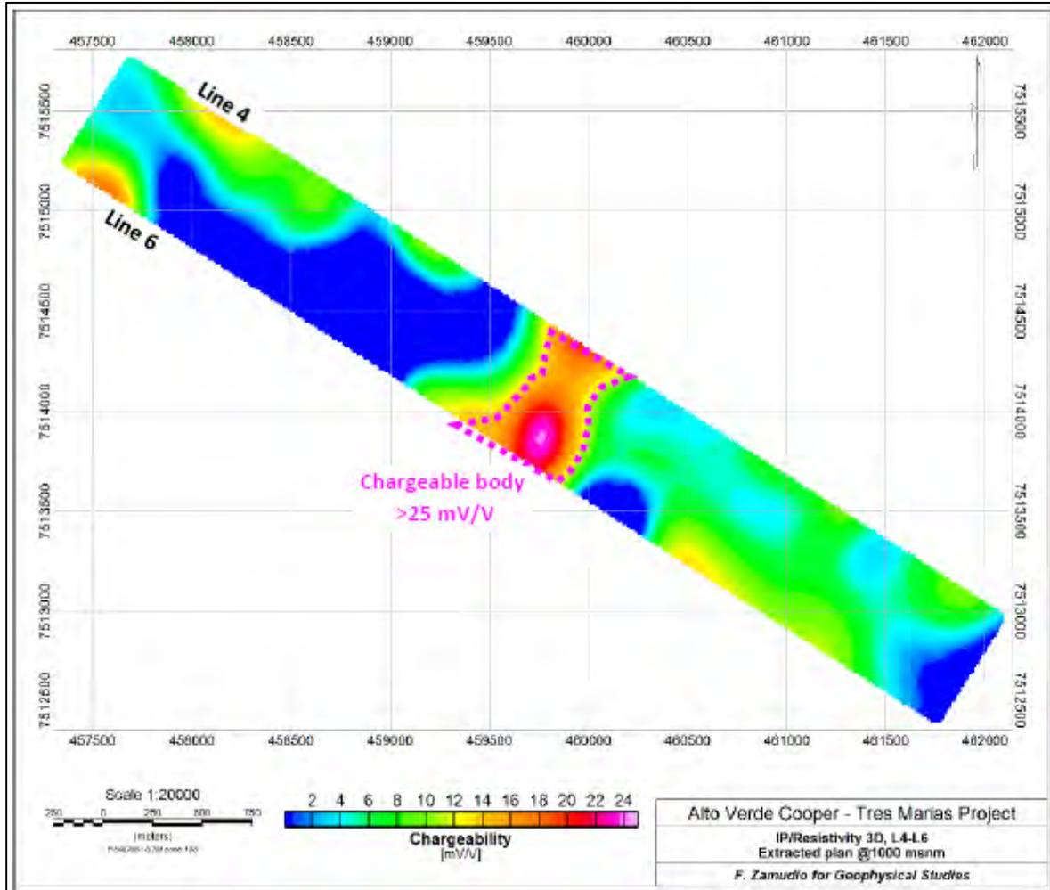
Figure 9-14. 3D-IP L4-L6 block (Western Target) with chargeability in plan view (“msnm” = m AMSL) (after Zamudio, 2021).
