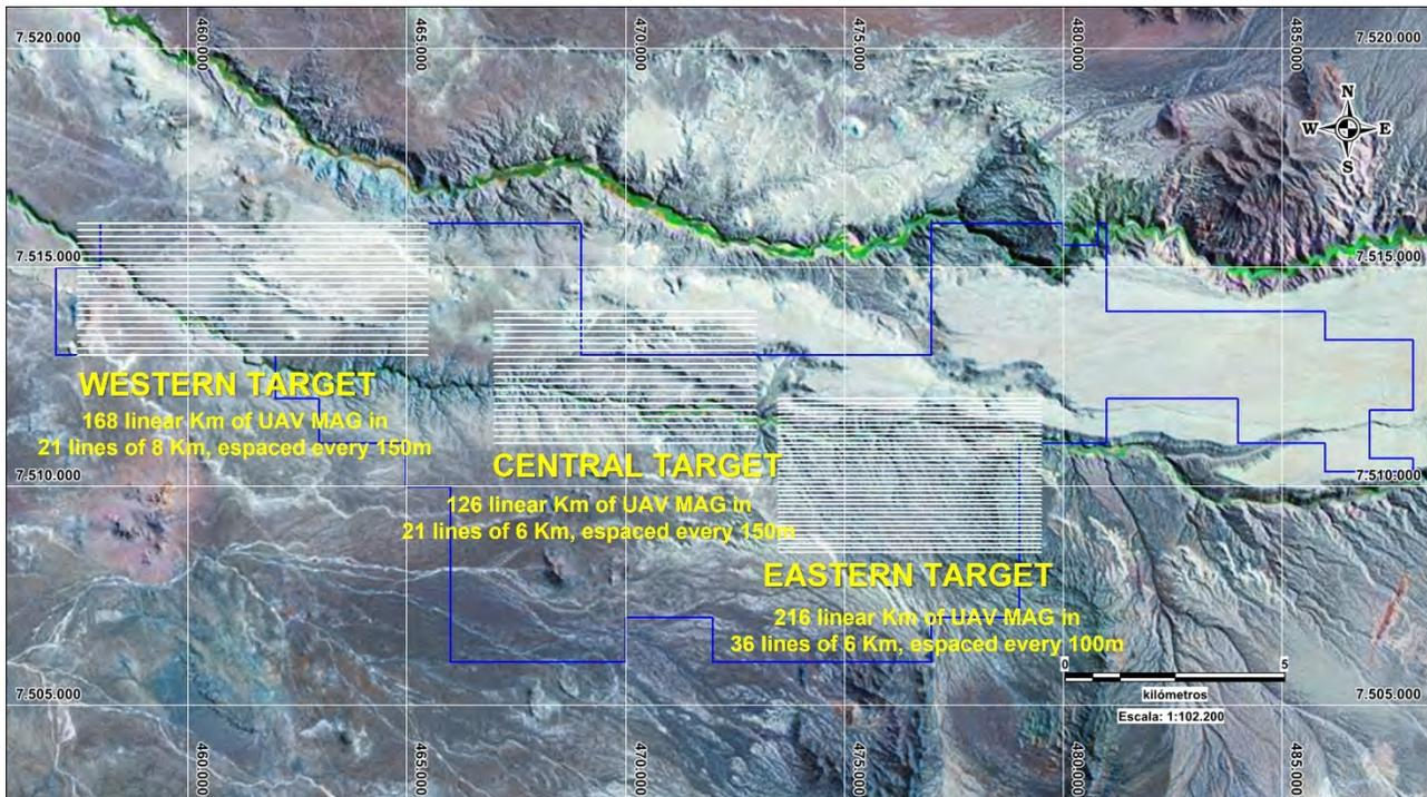
Figure 9-6. UAV magnetic survey over three target areas on the Tres Marías Copper Project (Alto Verde Copper, 2023).
