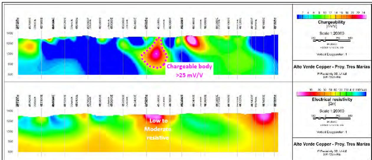
Figure 9-13. 3D-IP L4-L6 block (Western Target), chargeability (top) and resistivity (bottom), sliced at SW150m-NE (after Zamudio, 2021).
