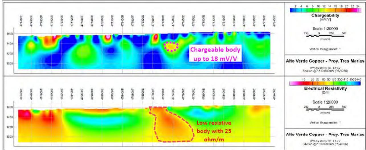
Figure 9-12. 3D-IP L1-L2 block (Eastern Target), chargeability (top) and resistivity (bottom), sliced at 7510600 mN (after Zamudio, 2021).
